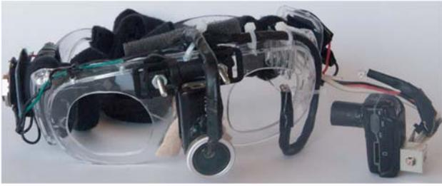
**Figure 1:** Our eye-tracking system costs approximately \$153 in off-the-shelf parts. The design centers around a pair of small, lightweight, point-of-view sports cameras, Veho’s Muvi Atom model, which record eye and scene videos.
