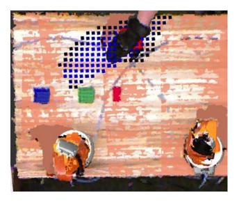
Fig. 2. Realtime visualization of a social force particle field generated from the user's motion patterns, rendered over point cloud data from the workbench sensors. Social force magnitude is represented by the blue channel, with the intensity of force increasing as particles range from black to blue. The estimated position of the user's hand is represented by a red square, shown under the gloved hand.
