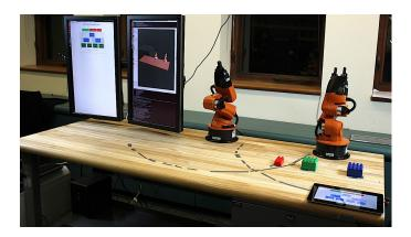
Fig. 1. The Collaborative Workbench used in the proof-of-concept implementation. The left monitor mirrors the tablet's display, showing live information about the task tree throughout task execution and allowing human participants to claim roles within the system. The right monitor displays a simulated environment mirroring the real world, along with social force fields as they are generated from user motion.
