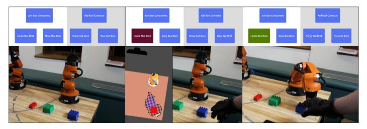
Fig. 4. An example of the "student" behavior, achieved by attractive social force. In the first panel, the robot is waiting for guidance before choosing an action. In the second panel, the user has gestured near the blue block, exerting social force in the goal region of "Locate Blue Block". The red box around the skill name indicates that robot intends to complete this action. The final panel shows the action as 'completed' in the task tree visualization (green box).
