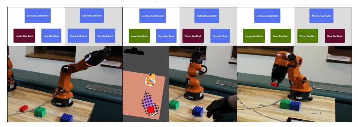
Fig. 5. An example of the "peer" behavior, achieved by repulsive social force. In the first panel, the robot intends to complete "Locate Blue Block". The second panel shows an interruption of the action by a human user. Upon detecting strong social force in its current skill's goal region, the robot aborts its execution and chooses a different, non-conflicting skill. The third panel shows the robot continuing to exercise conflict-avoidant behavior with the user.
