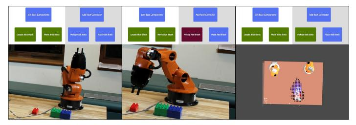
Fig. 6. An example of the "instructor" behavior, achieved by a using social force as a trigger. The first panel shows the robot evaluating available actions to teach. The second panel shows the robot demonstrating part of the "Pickup Red Block" subtask without actually completing it. In the third panel, the user has picked up the red block as previously pointed to by the robot, triggering the robot to mark the task as complete.
